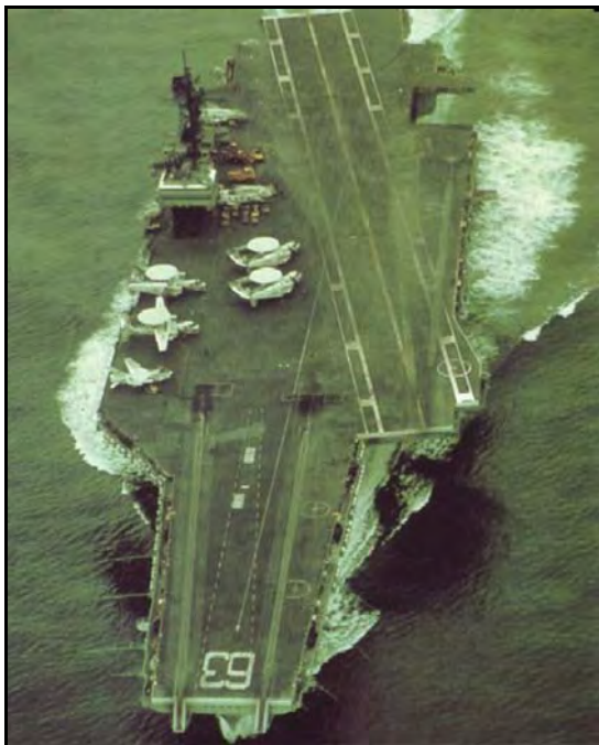
Fig. 150. Overhead view circa 1970s of Kitty Hawk showing her four catapaults – two at the bow and two at the waist on the angled deck. Also, note the area in the middle of the angled deck where the center line and ladder lines are well worn by aircraft during recovery when an aviator attempted to engage one of the four arresting wires with the aircraft's tail hook. The engaged wire pays out to its limits as the aircraft is "trapped" or decelerates while the engine(s) are pushed forward to full power to allow the aircraft to "go around" if the pilot fails to engage or "hook a wire." Each of the four steam catapaults was fixed with a Jet Blast Deflector ("JBD") which would be raised to deflect the jet exhaust from the aircraft while it was awaiting the catapault stroke. In this photo the JBDs are in their "down" or normal position as part of the flight deck. On the flight deck are four E2 Hawkeyes, one with the wings extended for flight and three with the wings folded; the massive radar domes are prominent. With the Hawkeyes is an A7 Corsair II, with folded wings. At the island and aft appear to be helicopters with the rotors folded.
